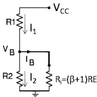
**Fig.1 Equivalent circuit for input resistance  $R_i$**
