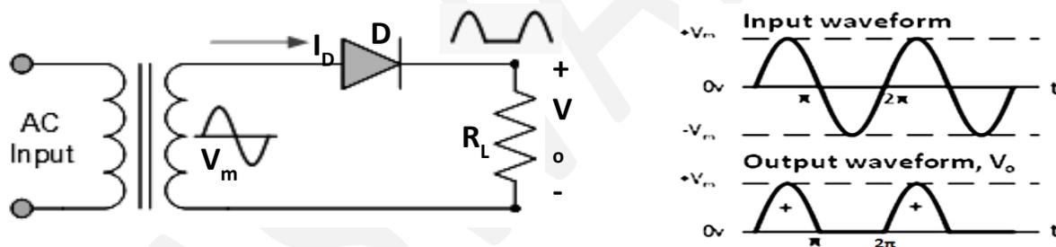
During positive half cycle of the secondary voltage  $V_m$ :
