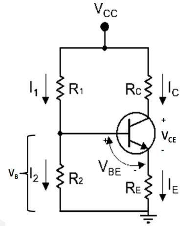
**Assumption:** The Base current  $I_B$  is very much smaller than the current  $I_2$ , through the resistor  $R_2$ .
