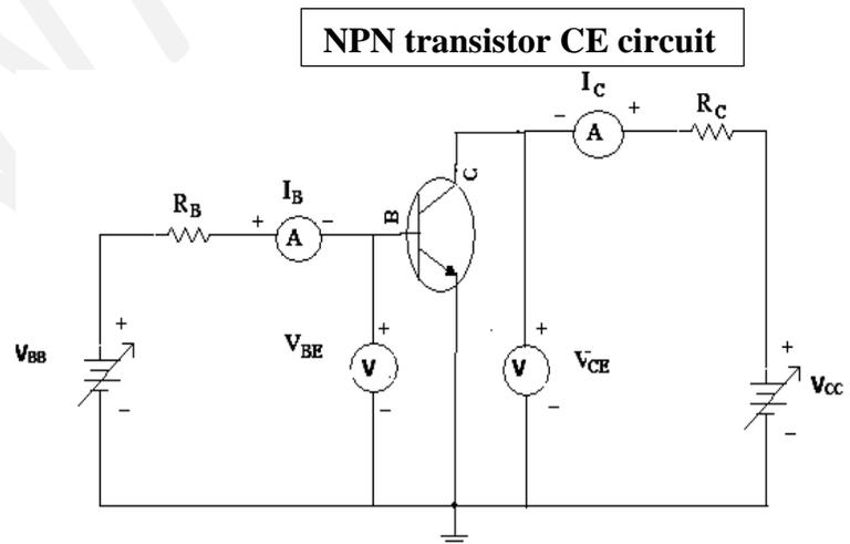
*Between cut-off and saturation regions normally transistor is employed for digital switch.*
