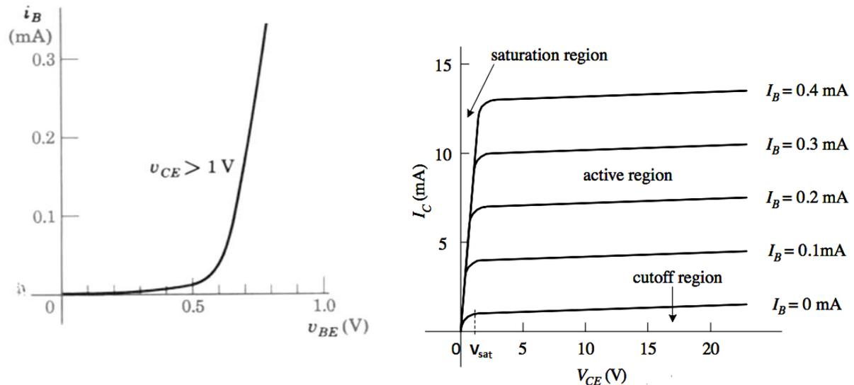
**Fig. NPN transistor CE configuration: (a) Input characteristics (b) output characteristics**
