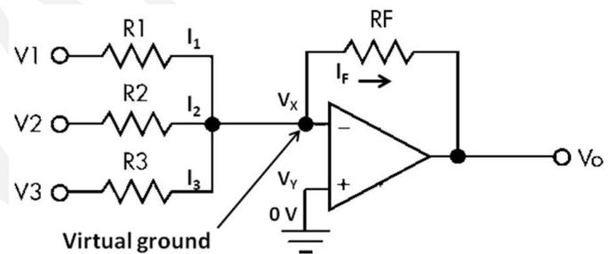
**Fig. Inverting summing op-amp circuit**
